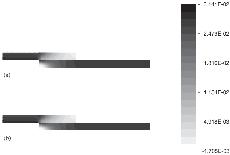
Fig. 12. Comparison of macroscopic \Sigma_{xx} (in GPa) contours by (a) continuum damage model and; (b) homogenized micromechanics.
